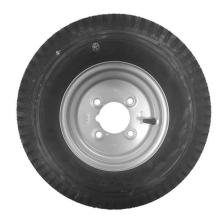
It is mandatory to ensure the minimum pressure indicated by the manufacturer in each case. The maximum tyre pressure permitted will be the lower of **4.9 bar** or the maximum pressure allowed for the tyre. The organisation has the right to check the tyre pressure at any time during the championship.
