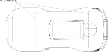
It will be necessary to enclose the exterior of the entire chassis; for this purpose any material described in point 4.3.2. of the regulations may be used.
