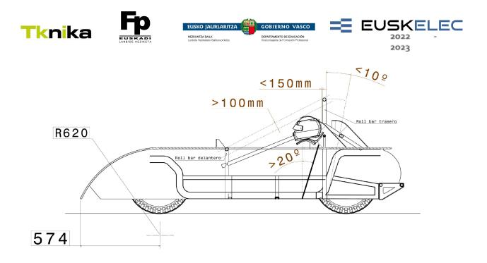
The roll bar can be installed by either welding or bolting to the chassis. Any bolts used must be **M8** or larger and the **quality 8.8** or higher. The front and rear roll bars must be connected by a sufficiently strong structure so that, in the event of an accident, the driver's compartment remains unaltered.
