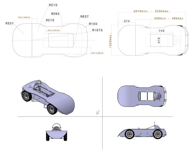
A drawing with the dimensions of the bodywork is attached.
